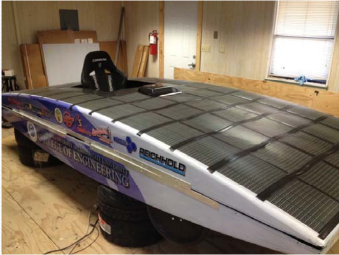
Solar Array Mounted
